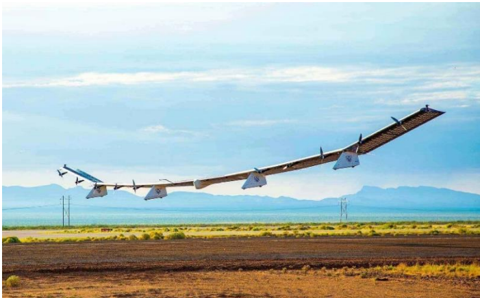
Sun glider, the unmanned aircraft system for HAPS developed by HAPSMobile (Reference)
