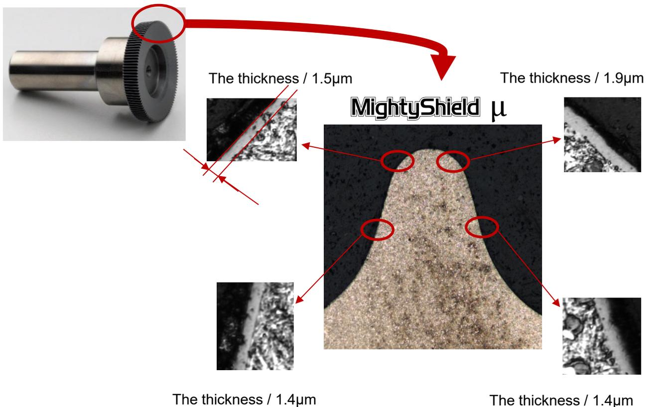
The thickness of the coating is formed as 2 $\mu$  or less, and the variation in the thickness from the tip to the root of the tooth is kept as 1 $\mu$  or less.
