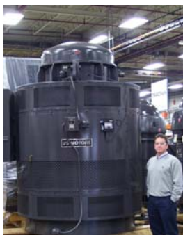
Titan Vertical High Thrust Motor (5,000 HP)
