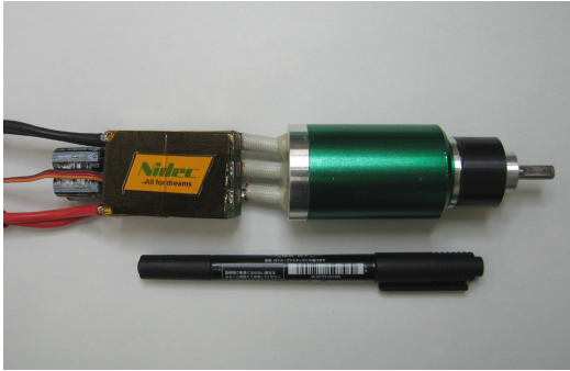
Figure 3 Nidec BDCM and Electronic Circuit Unit
