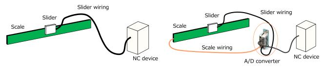
The electromagnetic induction method, the MPLW series' most prominent feature, possesses excellent durability that keeps detection accuracy from being affected by dust, oil, or condensation. Combined with other characteristics such as long and stable accuracy maintenance and thermal resistance based on a complete non-contact structure, this method is supported by various fields of industry.
