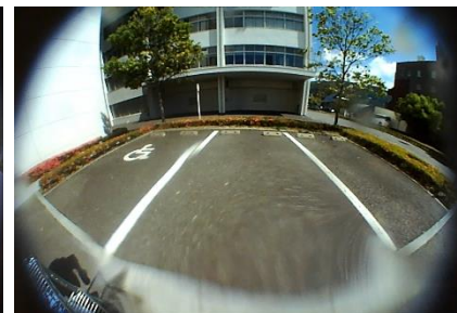
Camera, with hydrophilic coating, with water droplet (in a windless condition)
