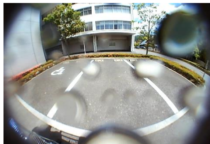
Camera, with water repellent coating, with water droplet (in a windless condition)
