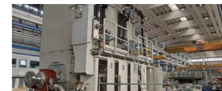
45MW hi-speed motor-generator
