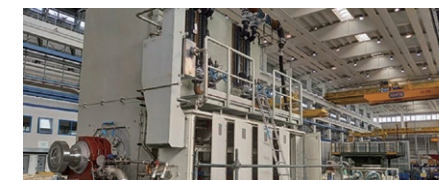
45MW hi-speed motor-generator
