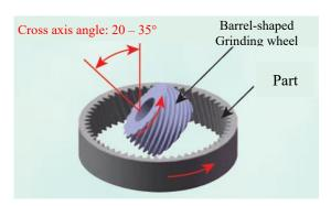
Process principle of internal generating grinding
