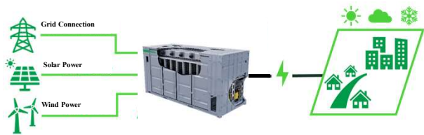
BESS(Battery Energy Storage System)
