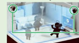
▲ A laser beam is irradiated from the lighthouse to reflect the user's location and movements in the VR
