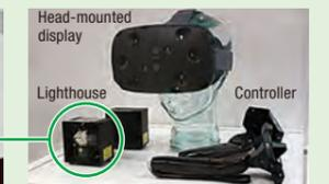
▲ VR kit. Nidec's FDB motor is installed in the lighthouse (a LIDAR device)
