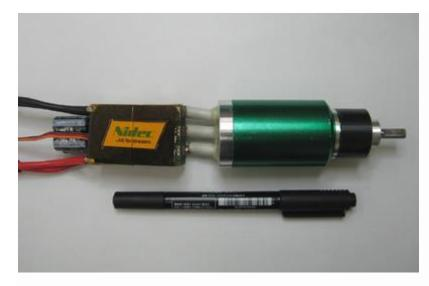
▲ F5B brushless motors and the Electronic Circuit Unit (ECU)
