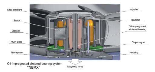
\*NBRX is an oil-impregnated, sintered-metal sleeve bearing unit developed from Nidec's NBR (Nidec Bearing Revolution) technology. NBRX uses lubricant oil highly resistant to heat and evaporation and is significantly less subject to wear. Strong vertical magnetic force maintains the spin axis orientation, enabling extremely low vibration in high speed rotation range.
